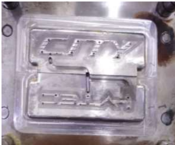
Suzuki Cover Splash Mould Double Cavity HPDC Crank Case 125 Rectification Localized by KTDMC
