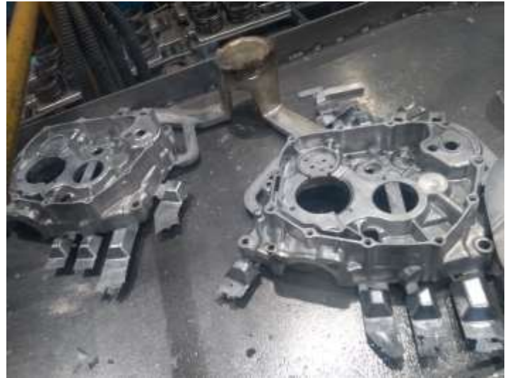
Suzuki Cover Splash Mould Double Cavity HPDC Crank Case 125 Rectification Localized by KTDMC
